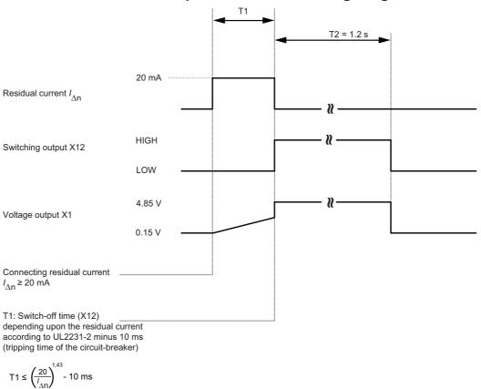
Fig. 2.6: Behaviour of the outputs when the values are outside the measuring range
