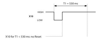
Fig. 2.4: Impulse duration for activating a reset
