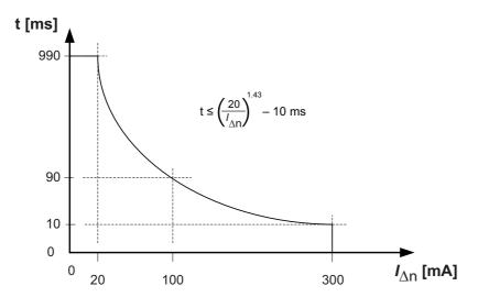
Fig. 2.7: Operating characteristics residual current monitoring module according to UL 2231-2
