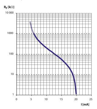
$$R_F = \frac{16\,\text{mA}\,x\,120\,k\Omega}{\text{I}-4\,\text{mA}} \,-120\,k\Omega$$
